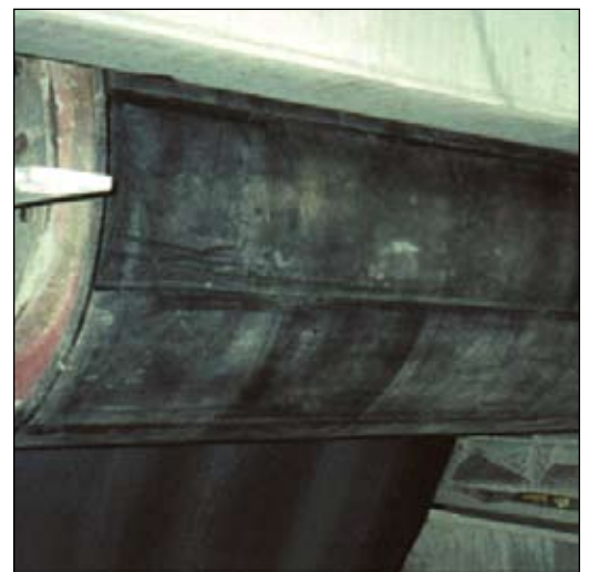
IMTECH ® NDP 60 pulley lagging extends the service life of pulleys in high abrasion applications.
