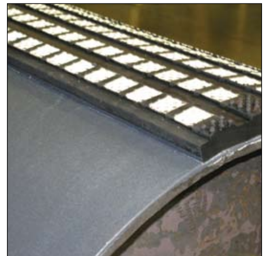
The specially formulated rubber compound adheres tightly to the pulley.
